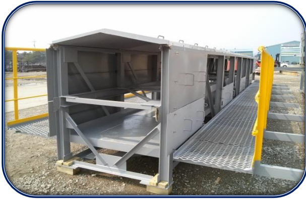
광양POSCO SNNC BELT CONVEYOR COVER포함전체조립납품
